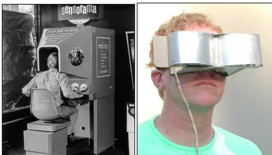
Figure 1 - The Sensorama (Left) and the Telesphere Mask (Right) by Morton Heilig.
