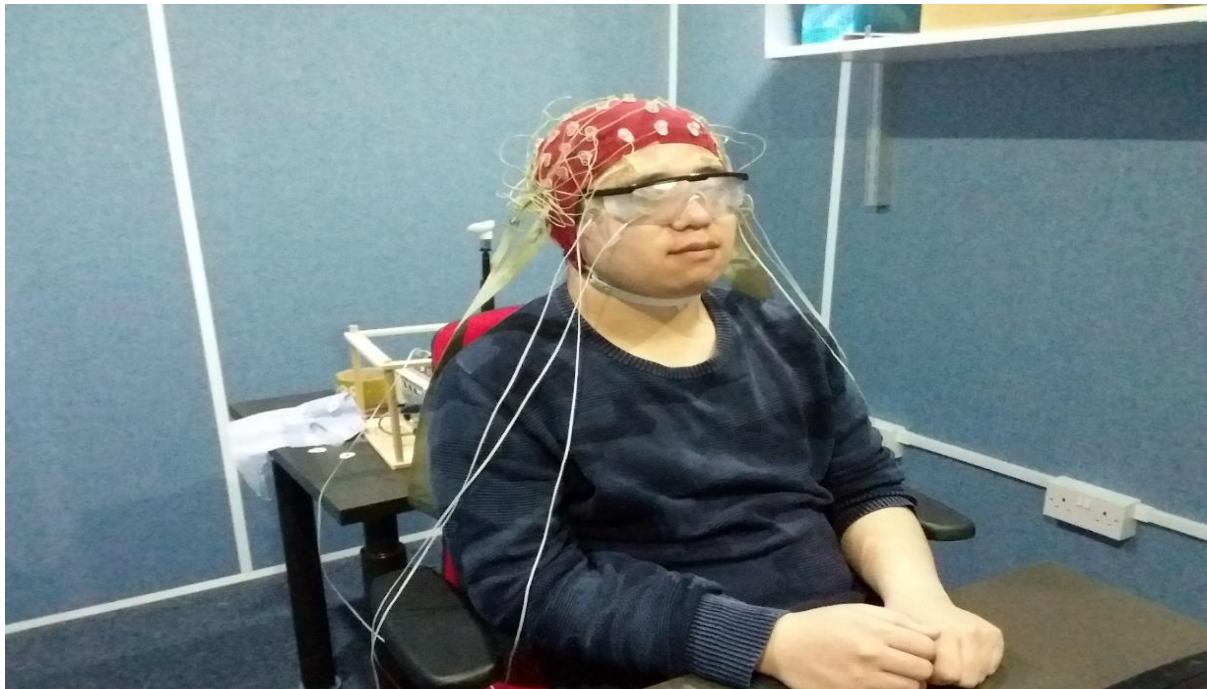
Figure 3.1 Subject is sitting in an electrically insulated and sound-attenuated room for the SSVEP recording experiment.
