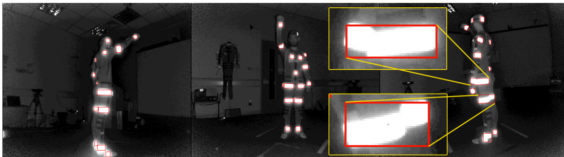
Figure 10. Reflector annotation using blob tracking on IR binary mask, visualized though on \mathcal{I}_{IR}^v IR data for the sake of better understanding. Erroneous estimates occur when reflector regions are merged.
