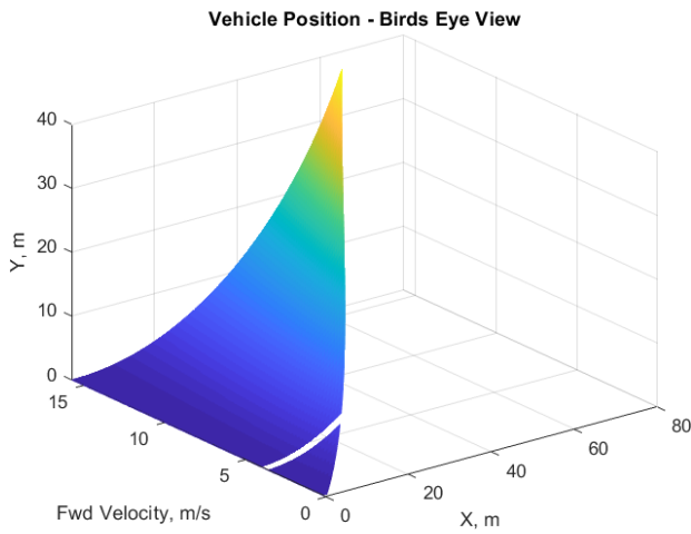
Figure 20: Vehicle position during a 3 degree corner, with varying velocity
