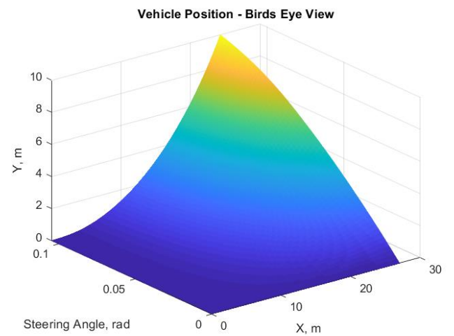
Figure 18: Vehicle position during a corner at 30mph, with varying steering angle
