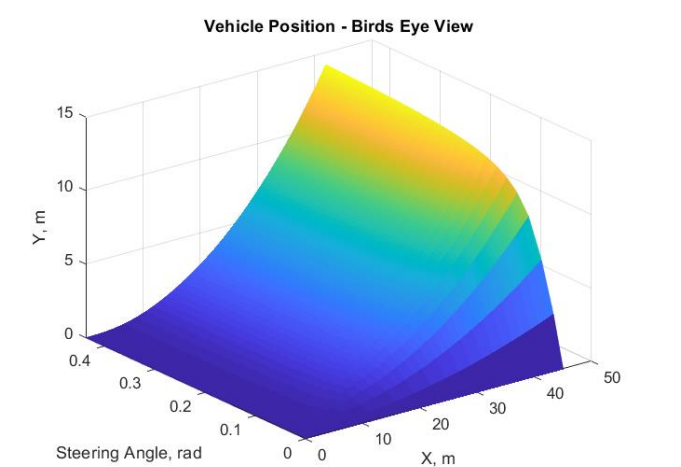
Figure 5: Vehicle position during a corner at 50mph, with varying steering angle
