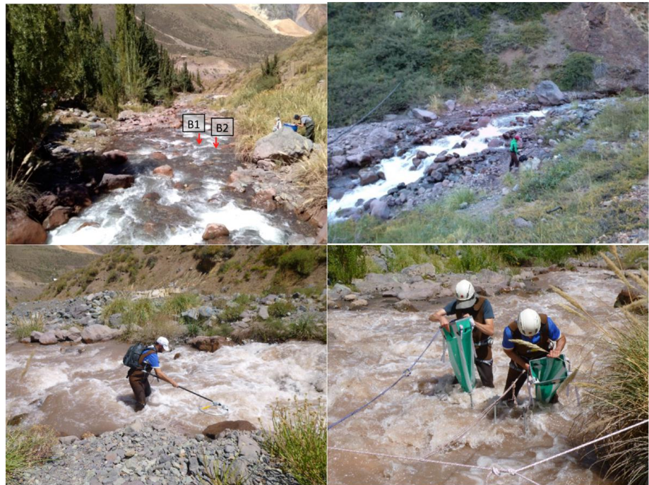
Figure 2. Views of the Estero Morales (a) at the monitored cross section; (b) at the upstream end of the reach where the PIT tracers were placed and surveyed; (c) during a PIT survey conducted with a portable antenna; and (d) during bed load sampling using Bunte traps. The channel width is about 7 m.
