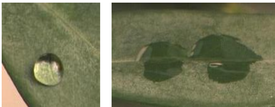
Fig. 30 A demonstration on a leaf surface of the addition of 5% w/w surface acting (wetting) agent using Polyacrylate liquid RM1 in water (right) versus the high surface tension of water (left).
